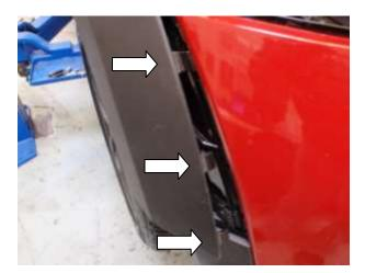
5. Pull the grill away from the bumper where indicated with arrows, you may need to apply some force so take care not to crack the grill or bumper. You now need to pull out the three clips holding the arch in position. From behind the bumper pull the clips towards the back of the car and push out.
