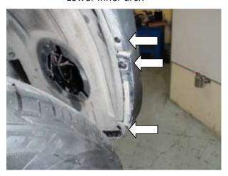
1. Park vehicle securely, jack the front of car and support on axle stands so that the front wheels are clear of the ground and raise bonnet. Starting on the driver's side turn steering wheel so the wheels are on full lock to gain access to the arch liner. Undo the 8mm screw, push out the pins from the three pin clips above using 2mm pin punch, then pull out the center of push clip using the flat bladed screw driver. Repeat this on the passenger side.
