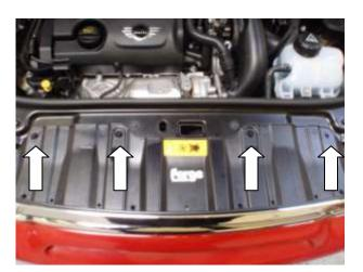
4. On the bottom of the bumper there are three more push in clips pull out the centers using the flat bladed screw driver then completely remove. Moving to the top of the bumper there are four 8mm screws holding the grill in position undo and remove these.
