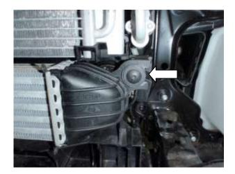
9. Undo the T25 screws holding the intercooler in place, undo the jubilee clamps and remove the intercooler.
